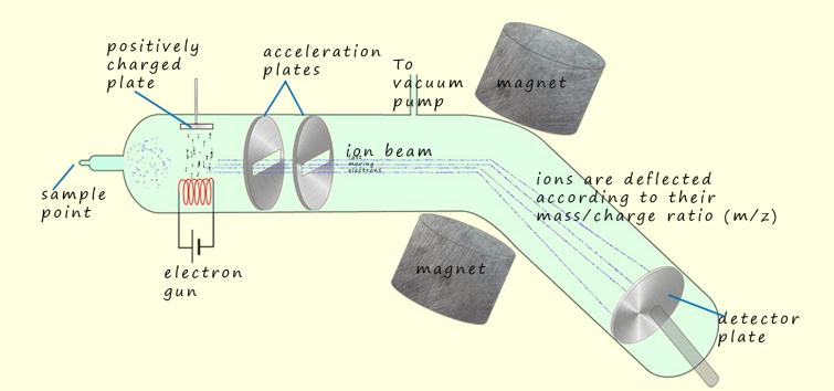
6. Sketch a basic diagram of a single beam mass spectrometer and label the key components.
